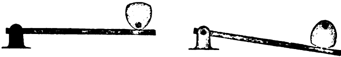
FIG. 8.—THESE REVOLVING CAMS TAKE THE PLACE OF THE WEAVER'S FEET, DEPRESSING THE TREADLES AS REQUIRED.
